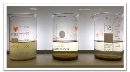
With conventional coagulant COD Removal:  $40\% \rightarrow 70\%$ pCOD Removal:  $50\% \rightarrow 90\%$
