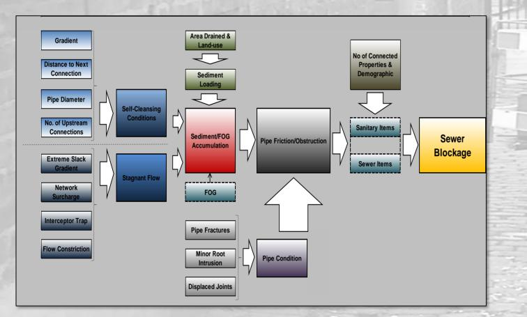
The initial conceptual model was developed based on the blockage formation mechanisms
