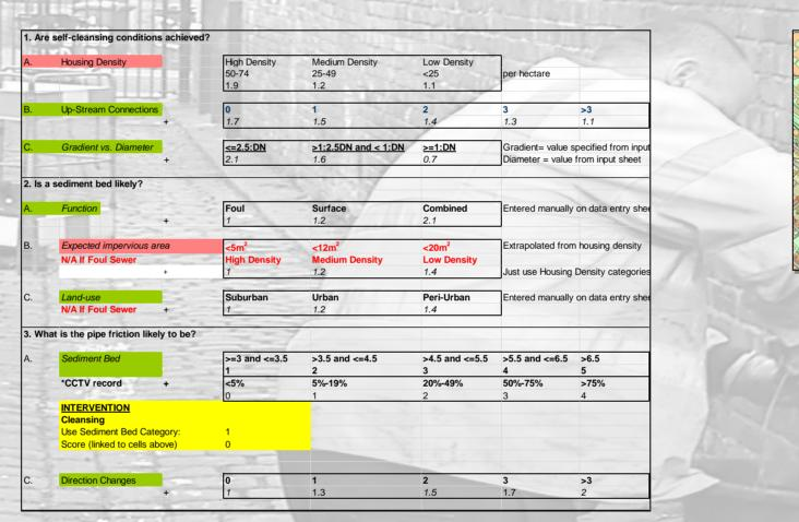
Each sewer parameter in the model was then assigned a score and developed into a scoring matrix
